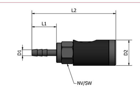
D1 ((mm) = Ø10 D2 (mm) = 26 L1 (mm) = 25 L2 (mm) = 88.5 SW (mm) = 21 Weight (g) = -
